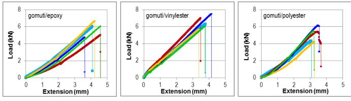
Figure 4. Load vs extension plots of tensile specimens
