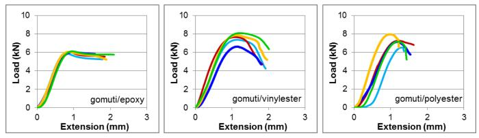
Figure 5. Load vs extension plots of compressive specimens
