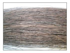
Figure 1.Unidirectional aligned gomuti fibre
