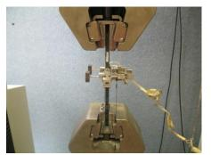
Figure 2. Tensile test set-up
