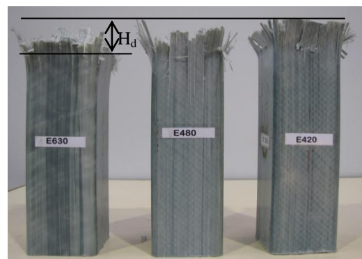
Fig. 8 Snapshot of collapsed tubes indicating damaged heights
