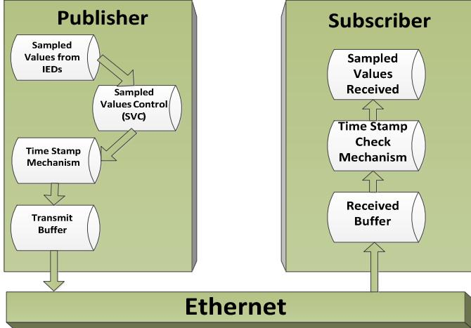
Fig. 2. IEC 61850 communications model for sampled value data.
