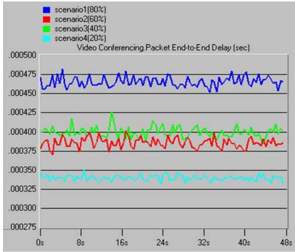
Fig. 7. Comparison of end-to-end *transmission delay* messages in different CPU background utilization.
