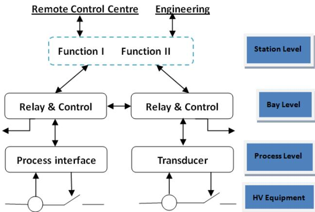
Fig. 1. Diagram of SAS hierarchy and logical interfaces.
