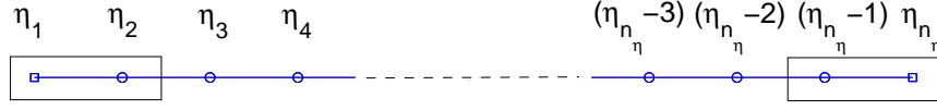
Figure 5.2: Special compact 2-point IRBF stencils for the left and right boundary nodes.
