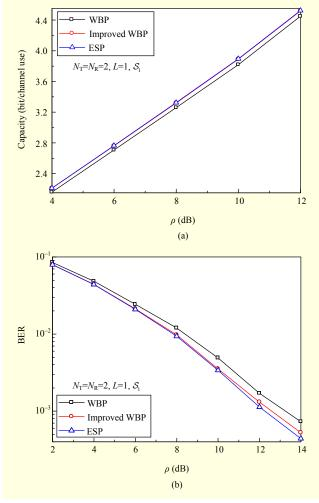
Fig. 2. (a) Capacity performance and (b) BER performance with  $N_T=N_R=2$ , L=1, and  $S_1$ .
