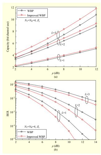
Fig. 5. (a) Capacity performance and (b) BER performance with  $N_T=N_R=4, L=1, 2, 3, \text{ and } S_3$ .
