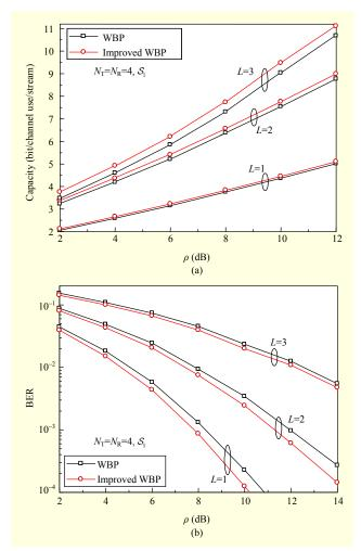
Fig. 3. (a) Capacity performance and (b) BER performance with  $N_T$ = $N_R$ =4, L=1, 2, 3, and  $S_1$ .
