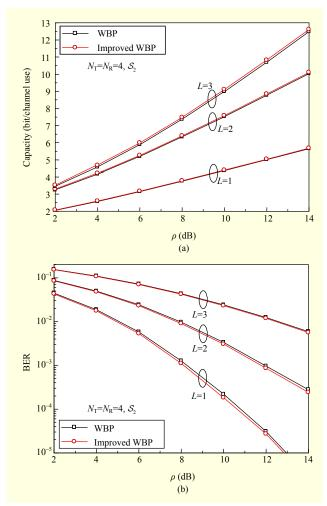
Fig. 4. (a) Capacity performance and (b) BER performance with  $N_T=N_R=4$ , L=1, 2, 3, and  $S_2$ .
