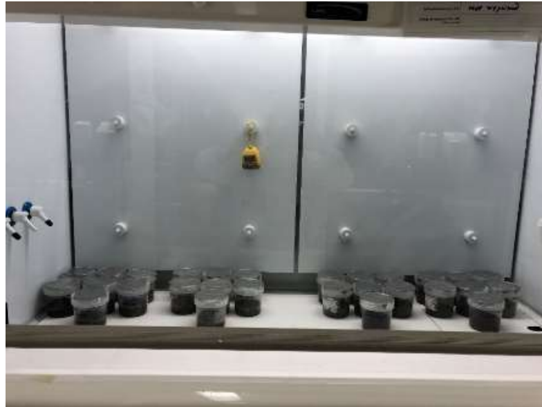
Figure 6.2: Containers containing Metham®-treated soil arranged in a fume hood for 19 days before the inoculation of fungal granules
