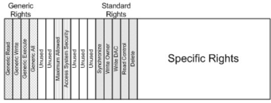
Fig. 4. NTFS Access Mask Layout
