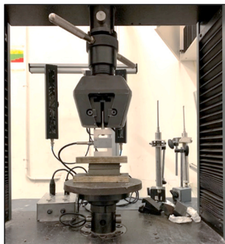
Fig. 3. Experimental setup for measuring the modulus of elasticity.
