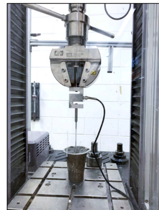
Fig. 2. Slow penetration test setup for SYS measurement.
