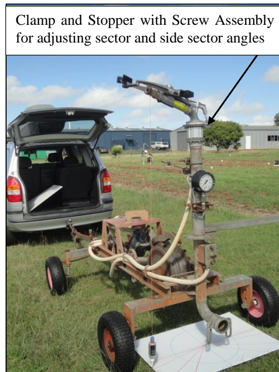
Figure 4-6: Large protractor drawn on plastic sheet to adjust sector and side sector angles.
