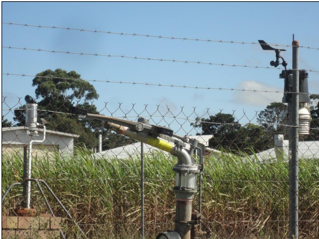
Figure 4-7: Three weather stations were used to measure wind speed and direction at the experimental site, and two close to the field site are shown here.
