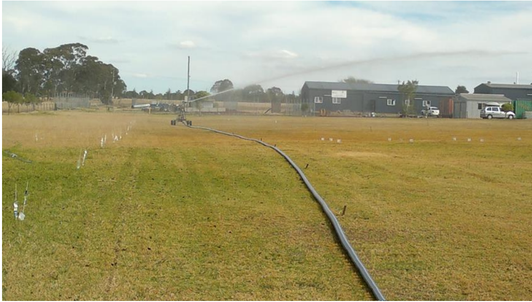
Figure 4-19: Photo of real experimental layout, while three lines of collectors were placed perpendicular to machine travel direction, using a sector angle of 180^\circ , and a side sector angle perpendicular to the travel direction, while the machine is traveling in curved movement.
