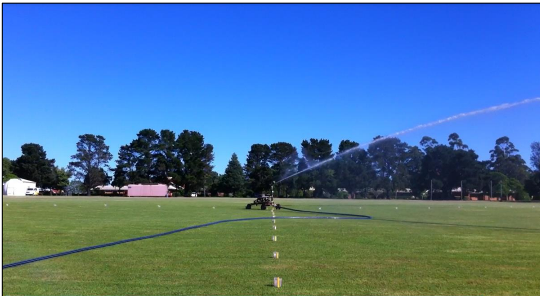
Figure 4-12: A photo of the irrigation machine and the four lines of collectors, setup for stationary tests.
