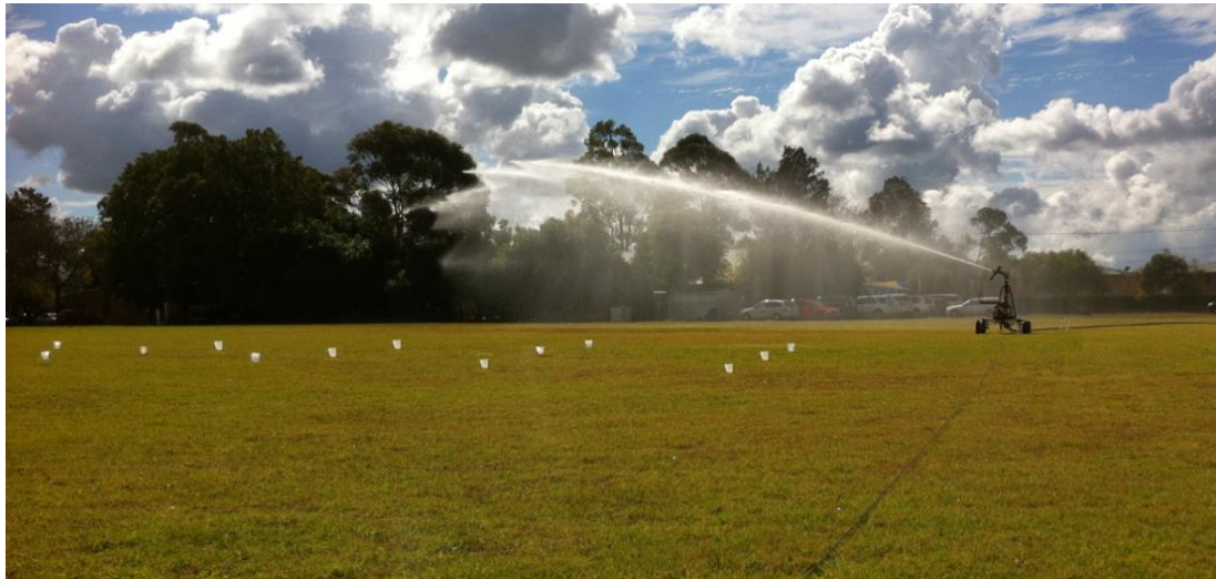
Figure 4-16 : Photo of the experimental field is shown with three lines of collectors placed perpendicular to the travel direction from one side of irrigated area by travelling machine.
