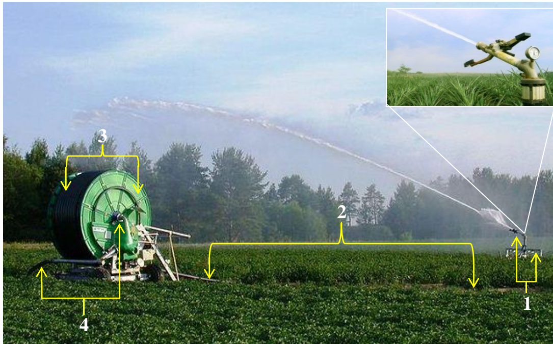
Figure 2-4: A travelling big gun sprinkler machine consists of a big gun on a cart wheel (1), distribution hose (2) and self-propelled stationary hose reel (3) and central pressurised supply water pipe (4) (Google Image, 2015) (Wade Rain, 2018)
