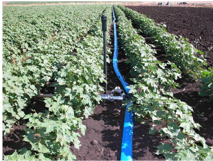
Figure 1. Hand shift solid sprinkler system used for application of irrigation water to the cotton crop.
