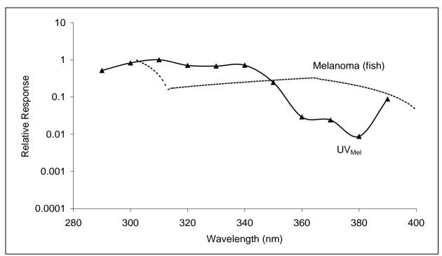
Figure 1. Fish melanoma action spectrum (Setlow et al, 1993) and the spectral response of the dosimeter.
