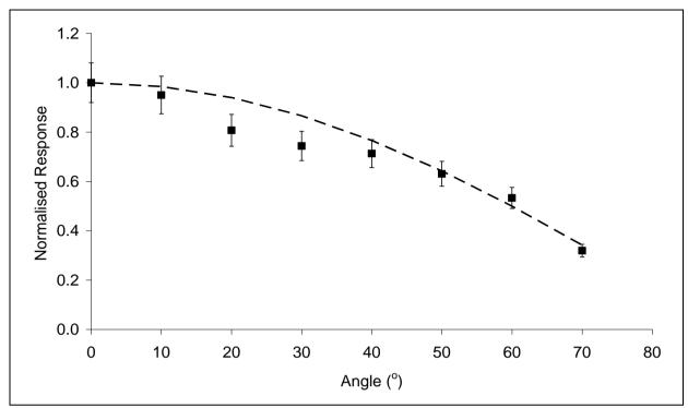
Figure 3. Comparison of the cosine response of the  $UV_{Mel}$  dosimeter to the cosine curve.
