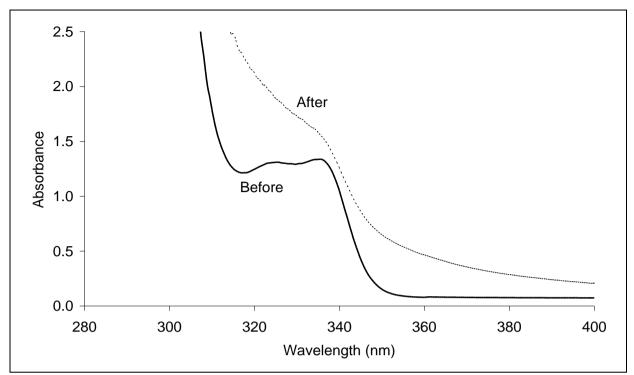
Figure 2. Before and after exposure absorbance characteristics of the  $UV_{Mel}$  dosimeter after a total  $UV_{Mel}$  exposure of 190 kJ/m<sup>2</sup>.
