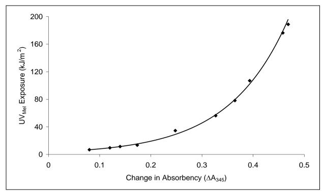
Figure 4. Dose response curve of the  $UV_{Mel}$  dosimeter for the measurement of the  $UV_{Mel}$  exposures.
