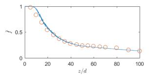
Figure 1: Centreline mean mixture fraction profile. MMC, line; experiment, symbol [14].
