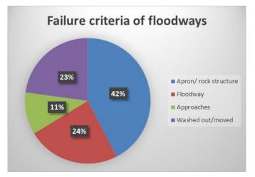
Figure 7: Floodway damaged due to different failure mechanisms
