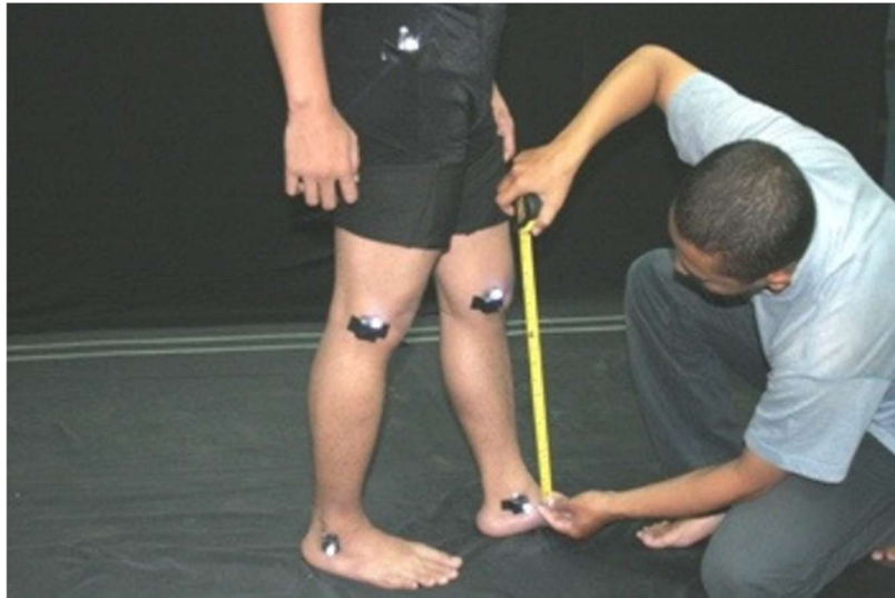
Figure 3.22: Calculating real measurement of knee-inner/outer ankle joint to be compared with photo measurement to obtain error difference (author's own image).
