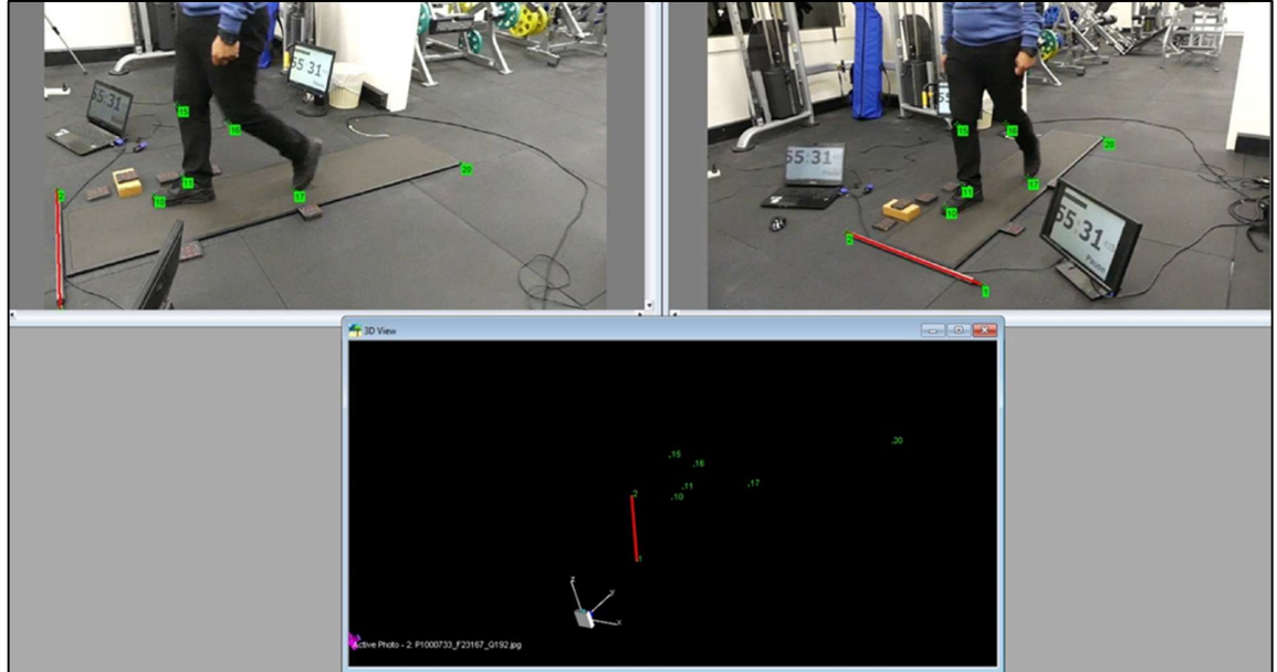
Figure 3.20: Capturing two images with clear view of the low-limb with the corresponding 3-D model of the points selected (author's own image).
