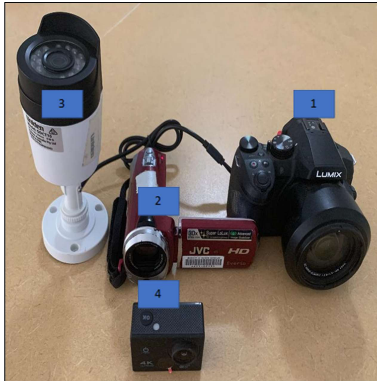
Figure 3.2: Four types of cameras used in this research. 1: Panasonic Lumix, 2: JVC handheld video camera, 3: Uniden CCTV camera and 4: Digital spy camera.
