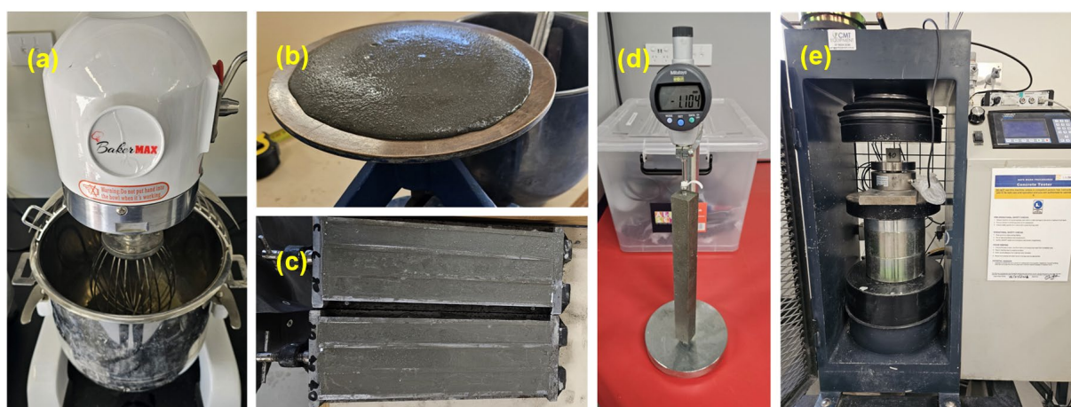
Figure 6. Specimen preparation and testing: (a) mixing of mortar; (b) flow table; (c) preparation of prism specimens for ASR expansion test; (d) measuring ASR expansion using vertical comparator; (e) mortar cube testing setup.
