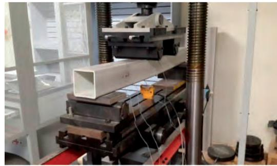
Figure 1. Experimental set-up for characterisation of elastic properties.
