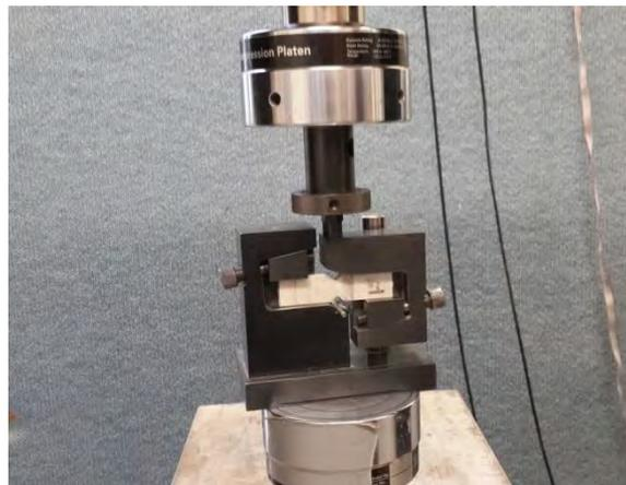
Figure C.1 shear test set-up
