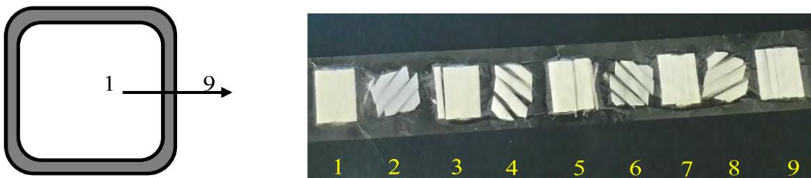
Figure B. 2 the orientation of the glass fibre
