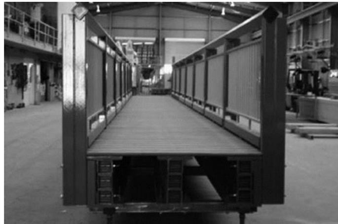
Figure 2.6 Footbridge fabricated from pultruded FRP tubes, Port of Airlie, Australia (<http://www.wagners.com.au>)
