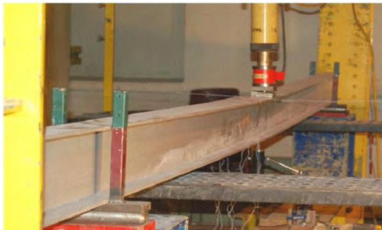
Figure 2.11 Lateral-torsional buckling of an I-shaped pultruded profile (Correia et al. 2011)
