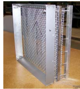
Figure 3. The frame used to hold screens in the wind tunnel (reproduced from Ranjit 2008)
