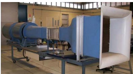
Figure 2. The wind tunnel (adapted from Ranjit 2008)
