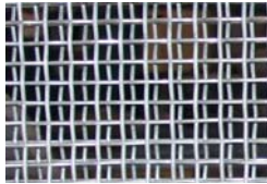
Figure 1. The cell size discrepancy of low-cost metal screen (reproduced from Ranjit 2008)
