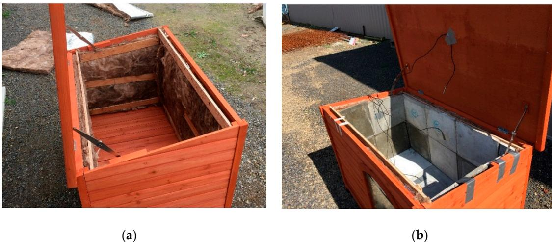
**Figure 2.** Test hut set up: (a) installation of insulation to the interior walls; (b) PCMCB installed on the interior surfaces.
