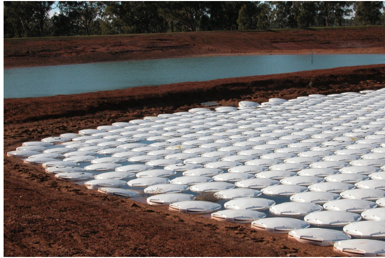
Figure 12 - Evaporation trial using (AquaCaps) circular design floating cover near Parkes, NSW
