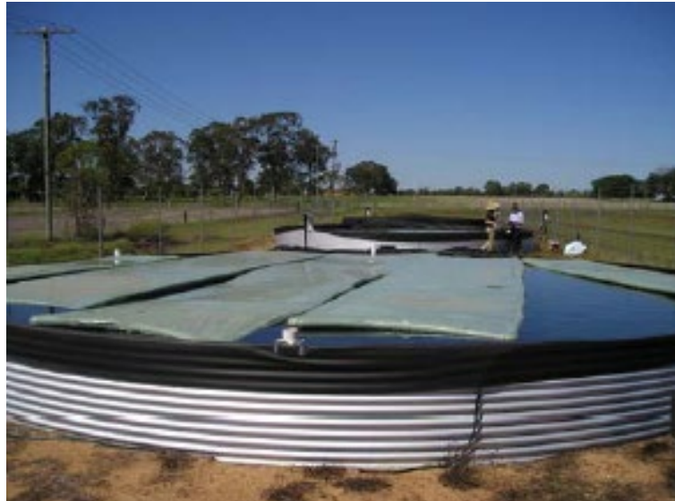
Figure 13 - Evaporation trial using prototype Raftex system of floating covers at USQ
