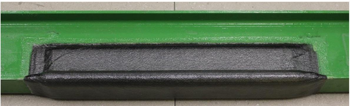
*Figure 6: Patch repaired beam with simulated 80% corrosion defect*
