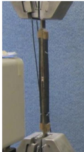
*Figure 7: Setup for tensile (left) and double strap shear joint (right) tests*
