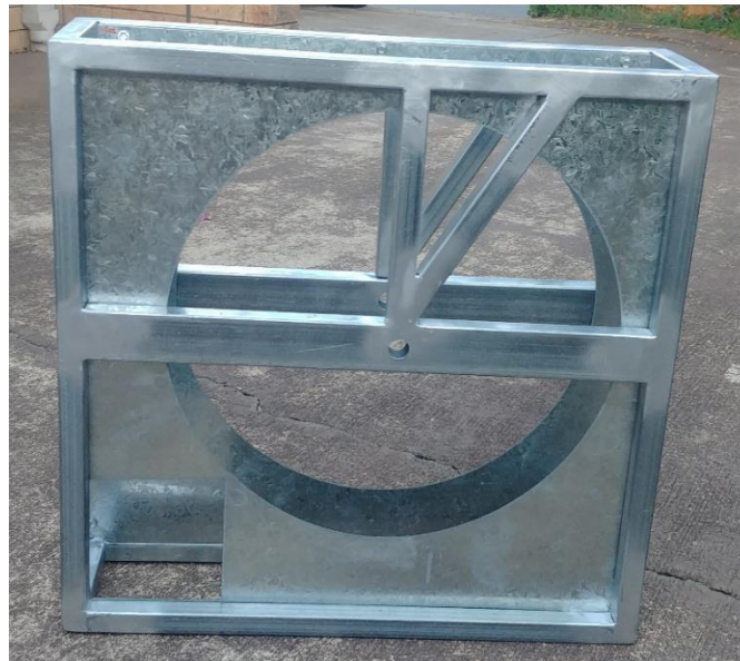
Figure 4.4: Desiccant wheel's cassette divided into four parts to form the required \theta_p/\theta_r ratio, and a square hole in the bottom left corner for the driving motor.
