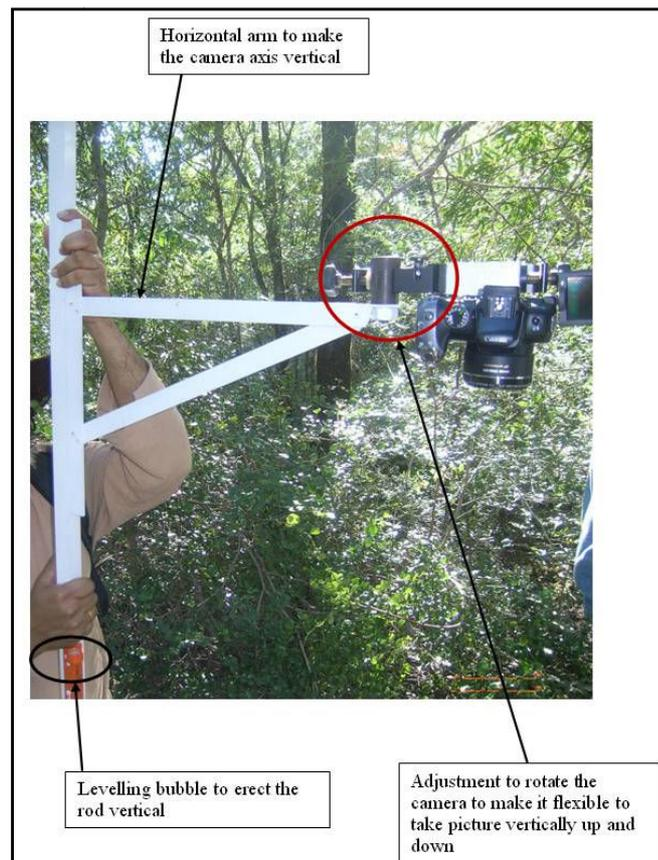
Figure 4: Set up of the camera.
