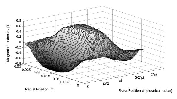
Figure 8: Output from Finite Element Analysis (Axial Flux Density)
