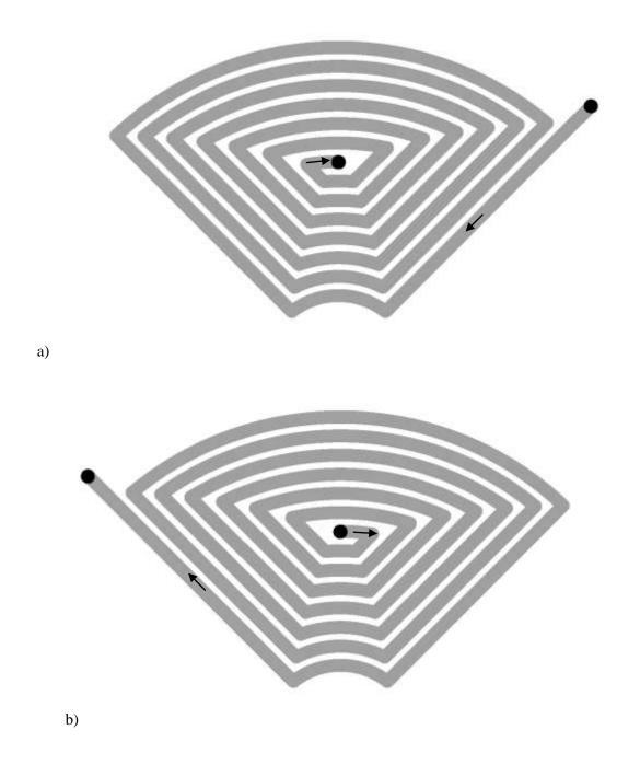
Figure 1: (a) Top Layer Spiral (b) Bottom Layer Spiral
