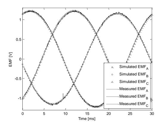
Figure 9: Phase EMF Waveforms (Test Motor No. 1, 1000 r/min)
