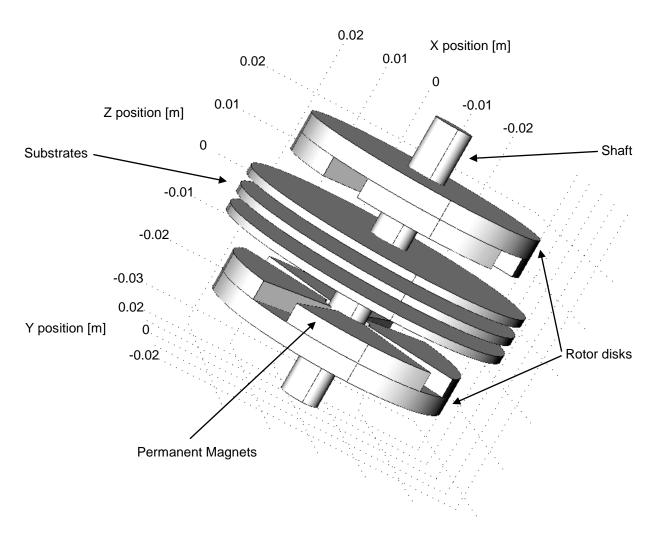
Figure 5: Exploded View of one of six Test Motors
