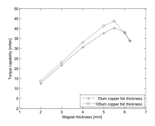
Figure 11: Torque capability versus Magnet thickness
