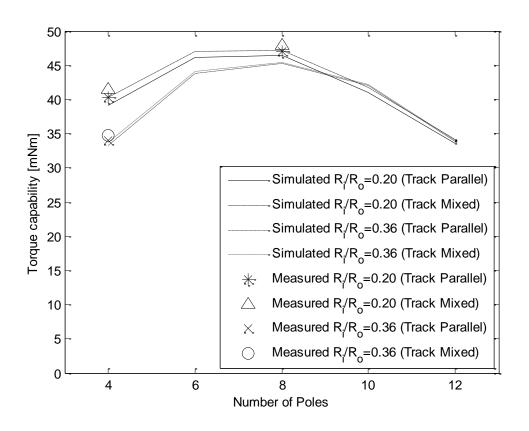
Figure 10: Torque capability versus Number of Poles
