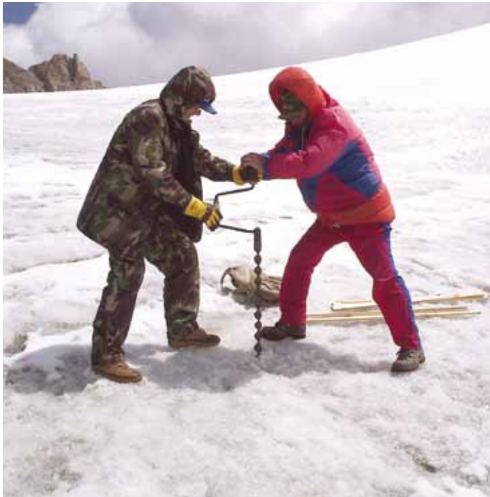
Pre-drilling of ablative measuring rods: Uzbekistan Hydro-meteorological Service
