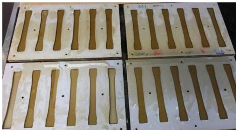
**Figure 3.2: Preparation of neat polyester specimens**
