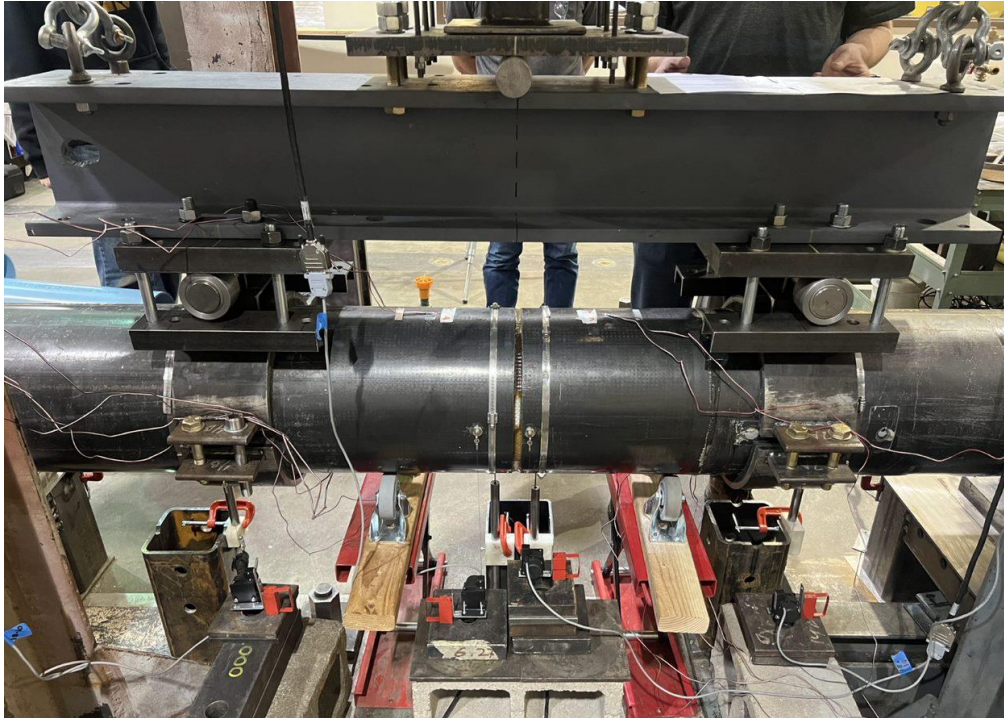
Fig. 16. Actual bending test setup, showing the positions of Linear Variable Differential Transformers (LVDTs) and strain gauges (CUB)
