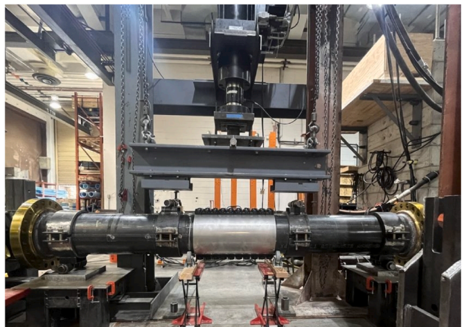
Fig. 2. Schematic view (left) and actual set-up (right) for lateral deflection test of SIRP systems (CUB).
