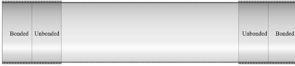
Fig. 14. A Schematic of the bonded and unbonded portions considered in the IRP system (Tien et al. 2023)
