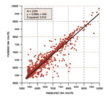
Fig. 2. Scatterplot of ANN-modeled and measured hourly cumulative raw counts of LWS 3 at Burmerange; data from April 13, 2007 to July 19, 2007 (Junk et al. 2008).
