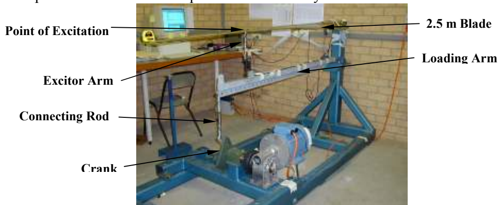
Figure 1 Fatigue test rig.
