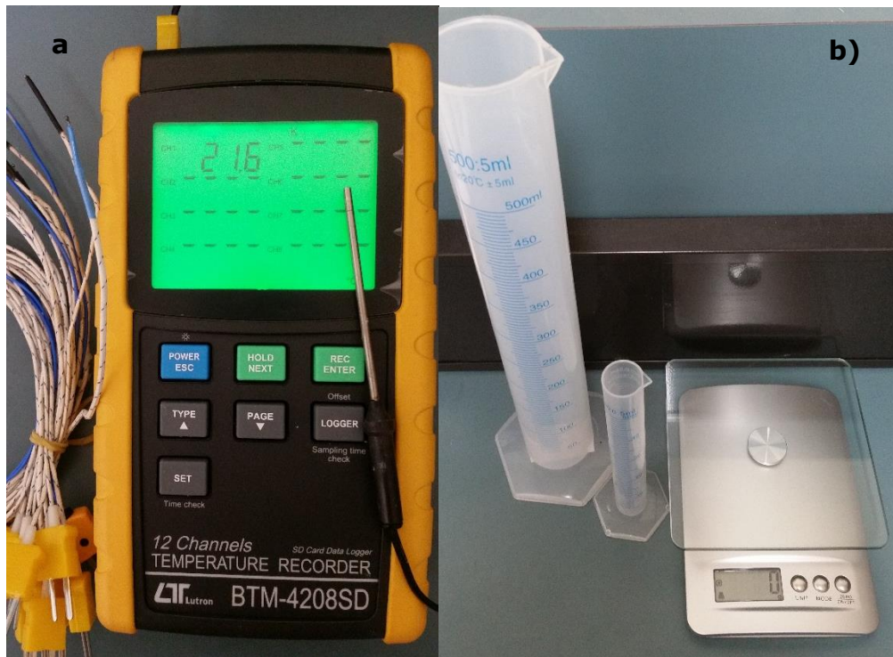
Figure 4. 6 a) the thermocouples and the data logger b) the measuring cylinders and electronic scale
