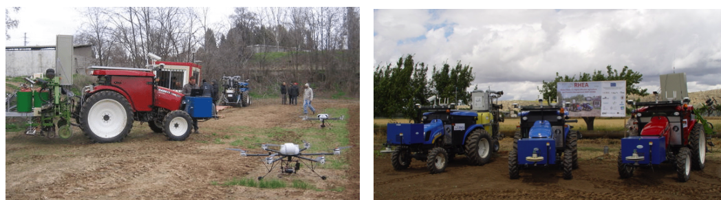
Figure 6. The RHEA project for pest control in cereal crops: Deployment of two rotor drones and three tractors working collaboratively for aerial inspection and ground level treatments (Left). Additional RHEA tractors used in a related pest control initiative (Right) [115].
