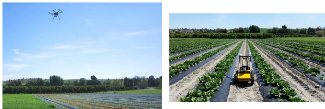
Figure 7. DJI 900 hexacopter manufactured by DJI, a leading technology company headquartered in Shenzhen, China, conducting an aerial survey over a lettuce field to capture multispectral data (Left). Husky UGV from Clearpath Robotics deployed at CPP's Spadra Farm for ground level support (Right) [116].
