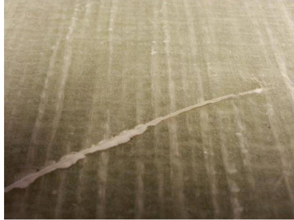
Figure 3-2: Silicon Doping of Optical Fibre at Ingress
