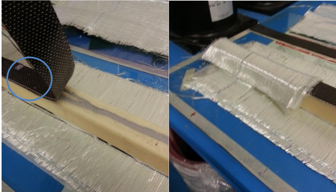
Figure 3-17: Beam Manufacture: a) Fibre optic cable recessed in core, b) Carbon and glass layers
