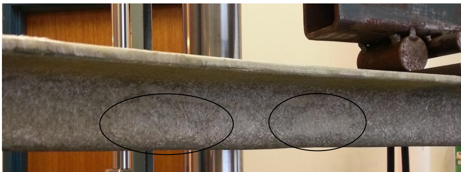
Figure 5-10: Early Signs of Fatigue in the Beams Outer CSM Layer
