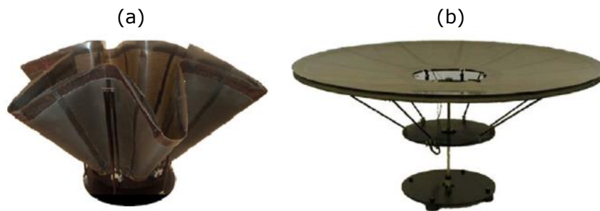
Figure 2.13: SMPC reflector: (a) Deformed shape and (b) recovered shape [120]
