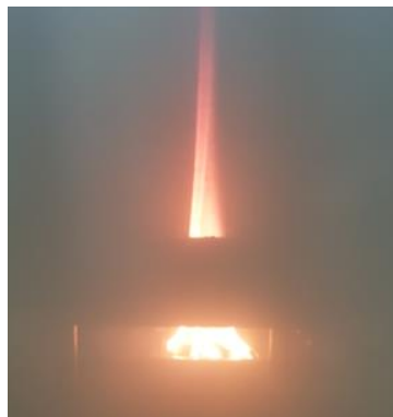
Figure 5.8: SMPC sample burning during a smoke density test
