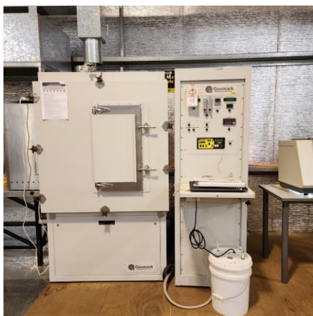
Figure 5.2: Deatak smoke density testing apparatus
