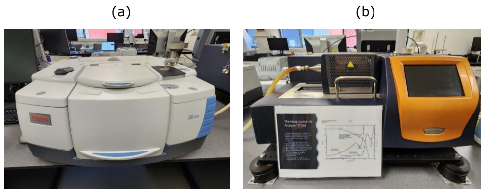
Figure 5.3: Apparatus used for TGA-IR testing; (a) FTIR and (b) TGA
