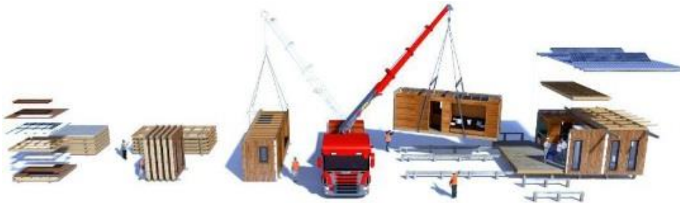
Figure 1.2: The process of prefabricated modular constructions [31]
