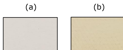
Figure 5.20: Colour of the neat SMP; (a) before and (b) after moisture exposure
