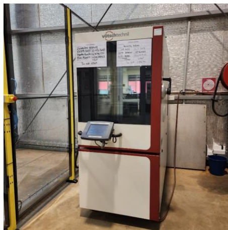
Figure 5.5: Moisture testing environmental chamber
