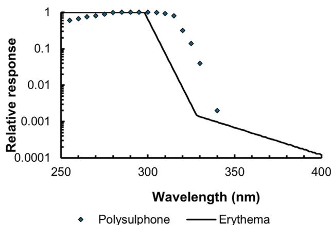
**FIGURE 1** Comparison of the erythema action spectrum<sup>19</sup> and the polysulphone spectral response.<sup>12</sup>
