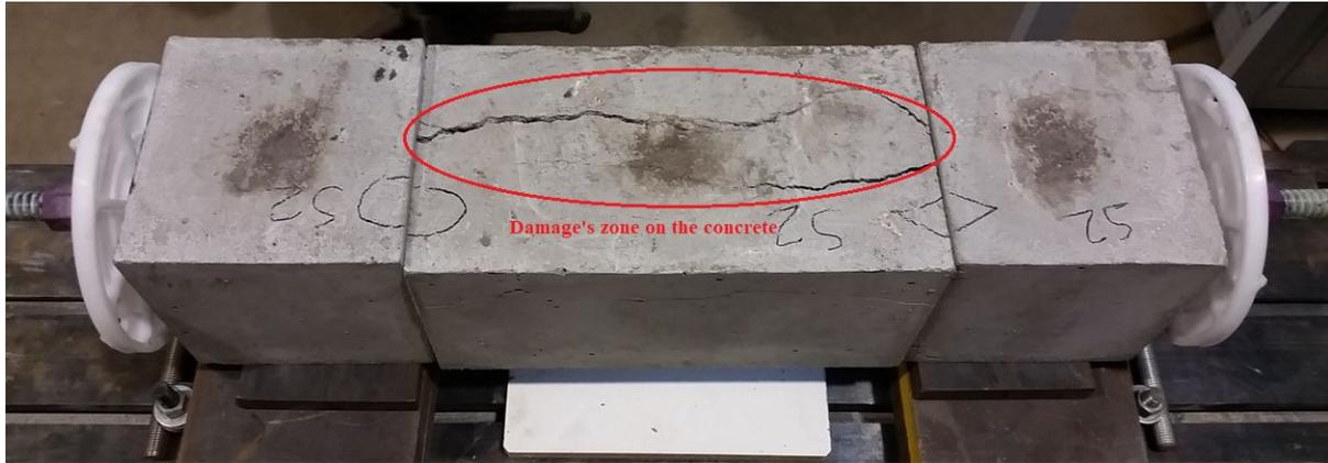
Figure 6: Severe damage resulting from a weak concrete matrix.
