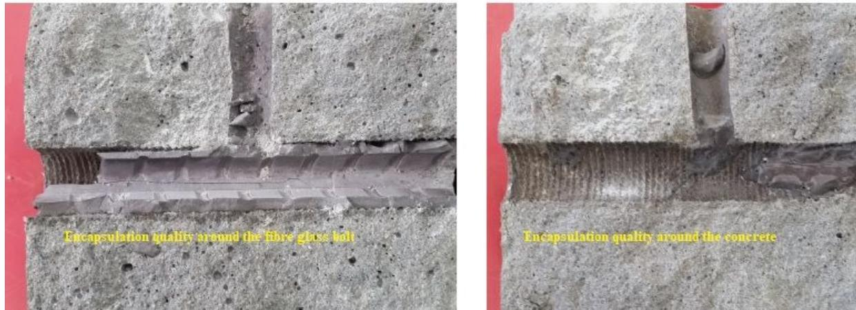
Figure 11: High quality encapsulation (left) around fibre glass bolt (right) around the concrete medium
