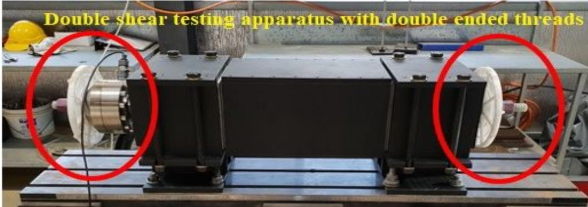
Figure 14: (Top) Illustration of fibreglass bolt geometry; (Bottom) Double shear testing apparatus with double ended threads
