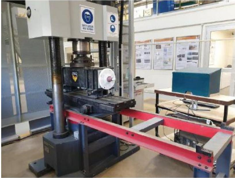
**Figure 1: Outline of SANS Machine used for double shear testing**
