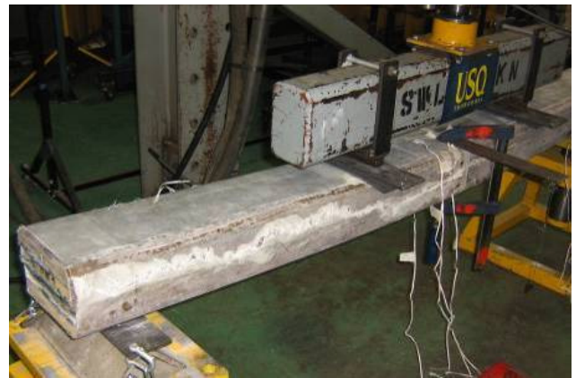
Figure 5. Sleepers made of LVL wrapped with triaxial glass fibres
