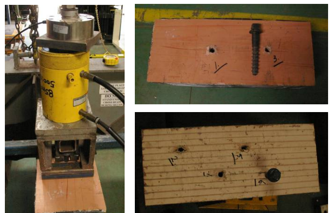
Figure 15. Test set-up and specimen for screw-spike withdrawal resistance
