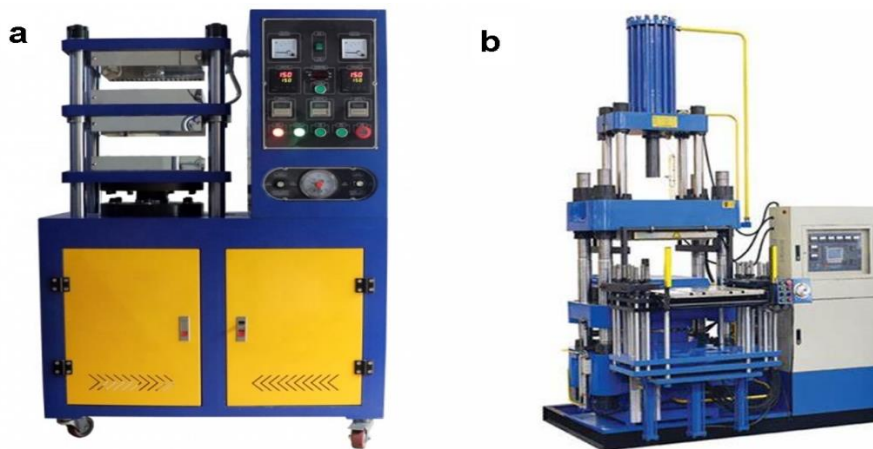
Figure 3.1. Images of flat vulcanizer. (a) Laboratorial and (b) industrial facilities.
