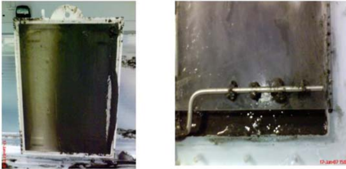
Figure 18. Left: Kubota membrane module partially scoured by biogas bubbles. Right: blocked diffuser located at the bottom of the SAMBR with only the far left hole remaining open for gas bubbles formation. Reproduced from (Trzcinski and Stuckey, 2009a).
