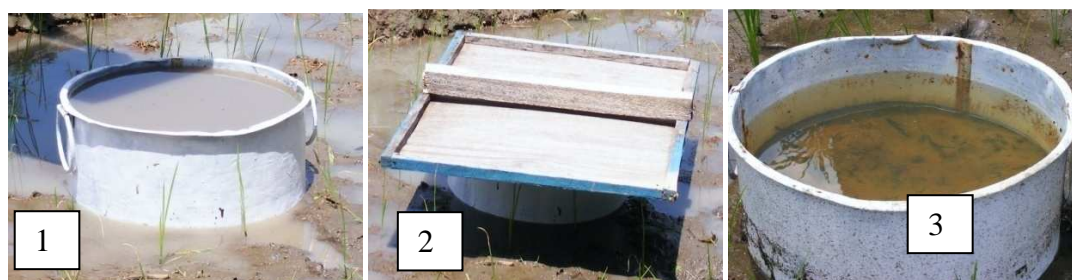
Figure 3.8 Covered metal cylinder installed just outside of the experimental plots for the measurement of daily percolation rates for the experimental site. 1, Cylinder just installed; 2, cylinder covered to minimise evaporation; 3, observing water depth in cylinder.
