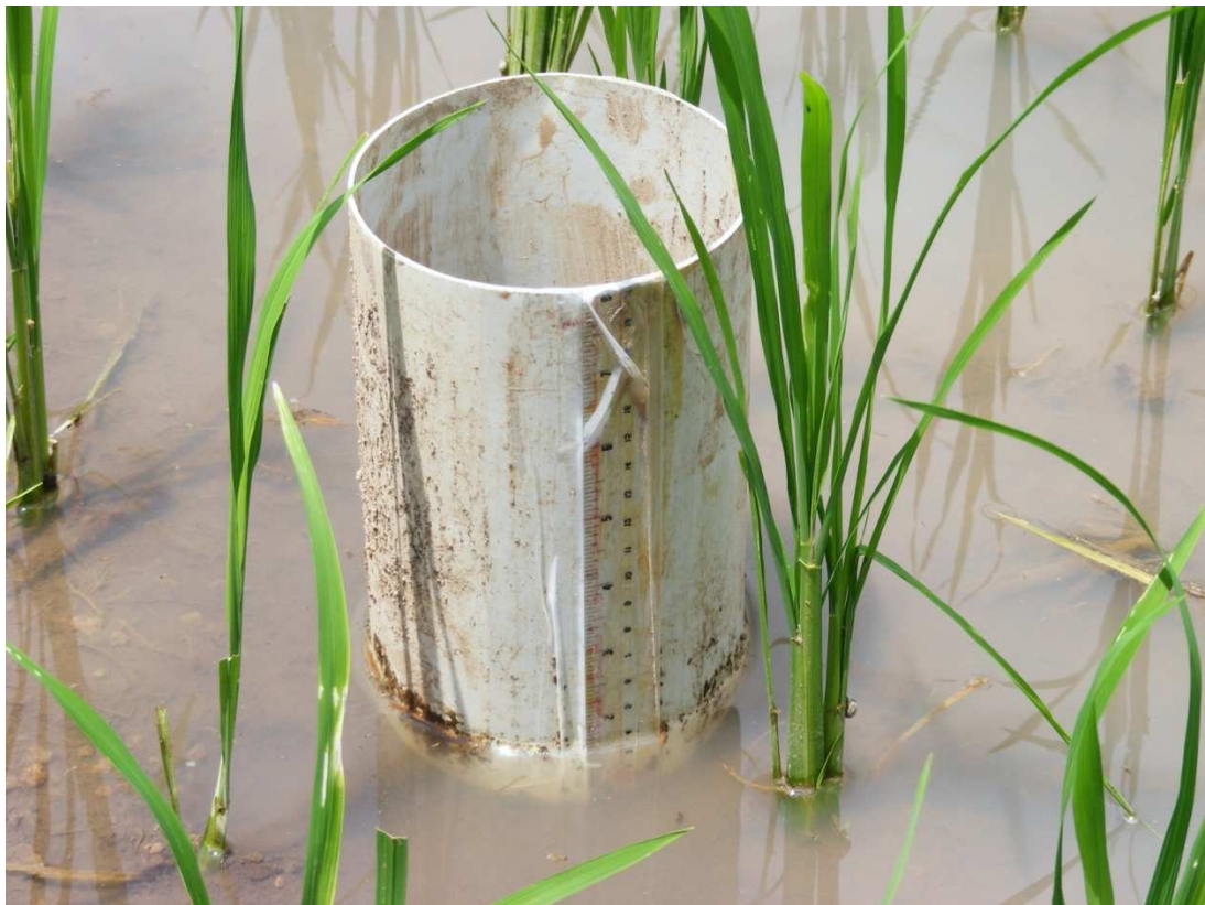
Figure 3.7 PVC pipes installed at all experimental plots to measure daily ponding depth and water depth below soil surface.
