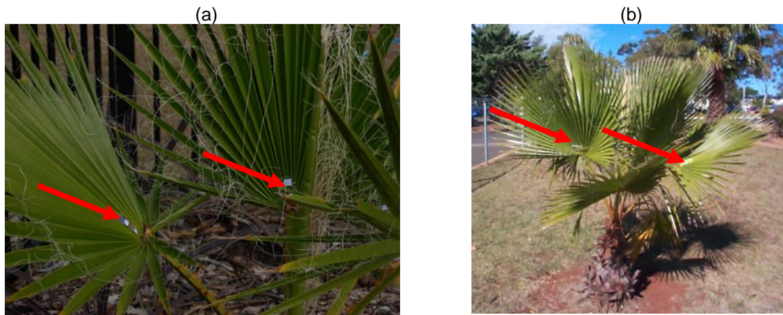
Fig. 1. (a) The miniaturised dosimeters attached to each leaf of a small plant in the field and (b) the long term dosimeters attached to a larger plant in the field. The dosimeters that are visible are marked with an arrow.
