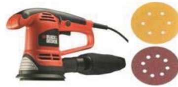
Figure: Orbital electric sander with 80 & 100 grit emery papers
