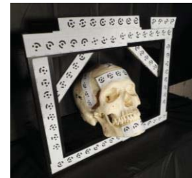
Image 1 – Model Skull being photographed with target control frame
