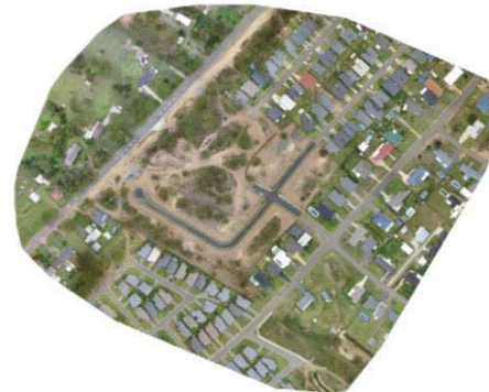
Figure 1 – Orthomosaic from UAV photos
