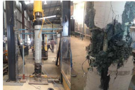
Figure 1. The compression test setup (l) and a tested specimen (r).
