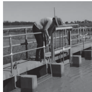
Figure 1 – The water levels measured by the pressure transducers in Channel B2/2, St George were manually calibrated
