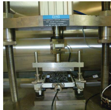
Figure 1: Indirect tensile strength (Resilient Modulus Test).
