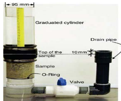
Figure 1: A picture depicting the Falling Head Test Apparatus
