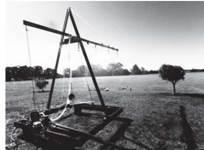
Figure 1: Makeshift mobile sprinkler rig used for model evaluation.
