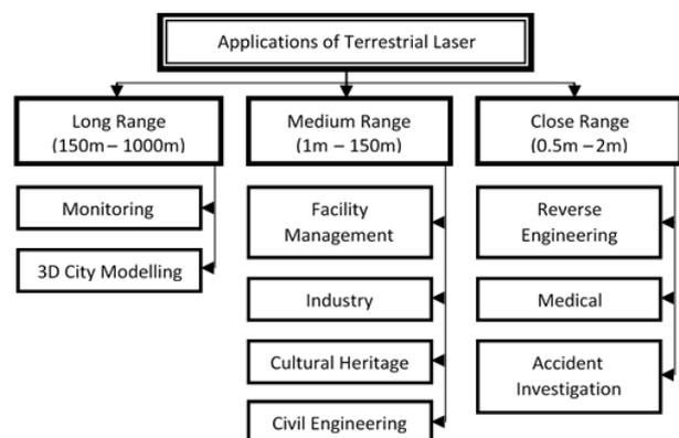
Figure 1. Classifications of TLS based on range mechanism [1]
