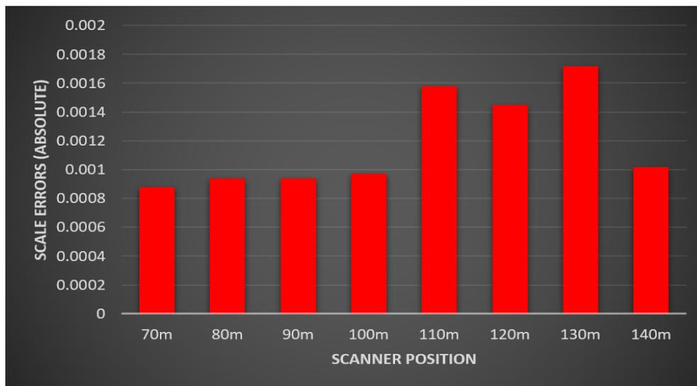
**Figure 10.** Scale errors for multi distances configuration
