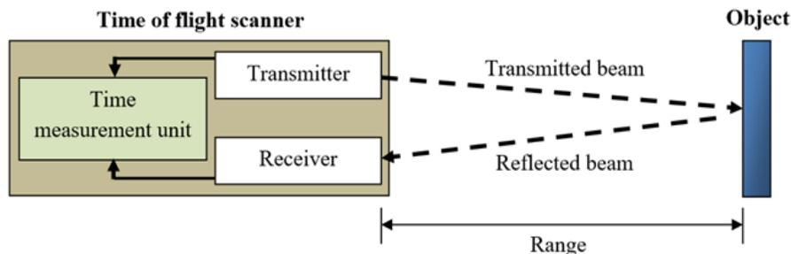
Figure 2. Mechanism of time of flight scanner
