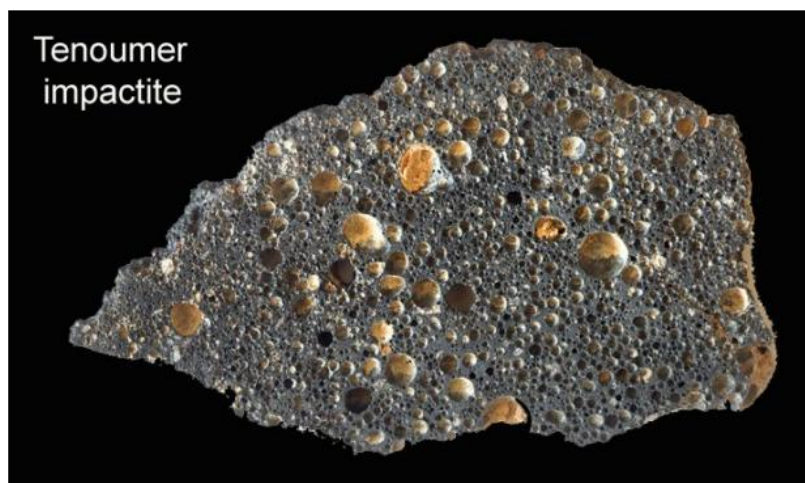
Figure 2.19: A 4-inch wide slice of shock-melted glass from the Tenoumer Impact Crater in Mauritania, Africa ( http://astrobob.areavoices.com/tag/coesite ).
