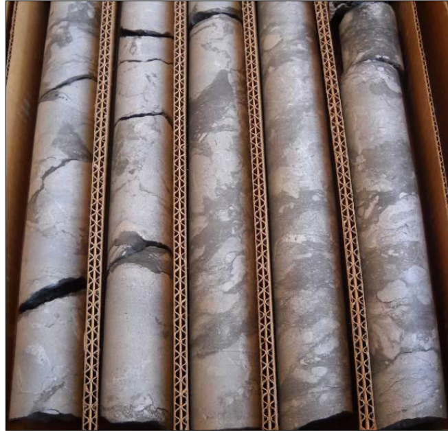
Figure 4.58 Sample of drill cores from the USGS Flynn Creek Crater Drill Core Collection in Flagstaff, AZ. (after Hagerty et al., 2013).
