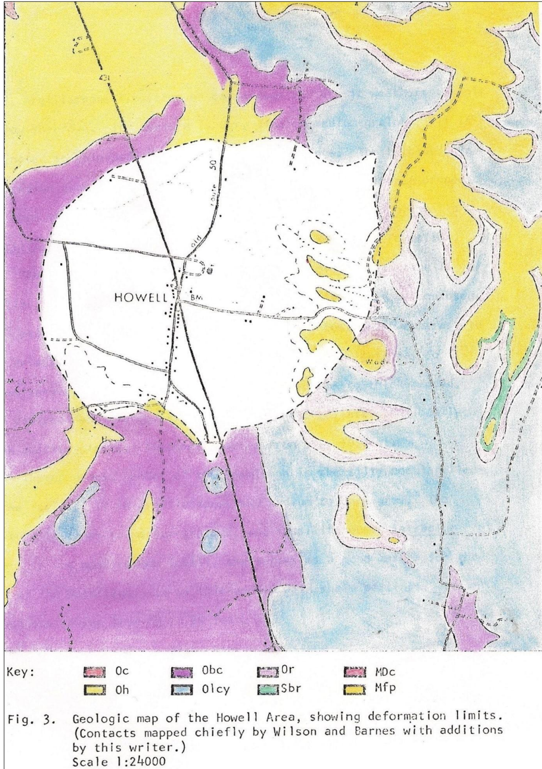
Figure 4.72: A geological map of the Howell area as mapped by Wilson and Barnes and with additions by Woodruff. [Key: Oc = Carters Limestone (Middle Ordovician), Oh = Hermitage Formation (Middle Ordovician), Obc = Bigby-Cannon Limestone (Middle Ordovician), Olcy = Leipers Formation and Catheys Limestone (Middle and Upper Ordovician), Or = Richmond Group (Upper Ordovician), Sbr = Brassfield Limestone (Lower Silurian), MDc = Chattanooga Shale (Upper Devonian and Lower Mississippian), Mfp = Fort Payne Formation (Lower Mississippian)] (after Woodruff, 1968).
