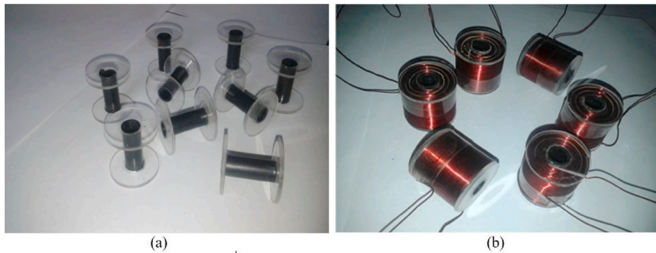
Fig. 3. Electromagnetic design: (a) bobbin, and (b) electromagnets.
