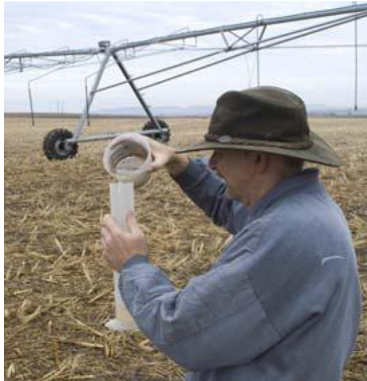
Figure 2.2: Measuring the volume of water in a catch-can using measuring cylinder (source: Smith, Cotton CRC Water Team)
