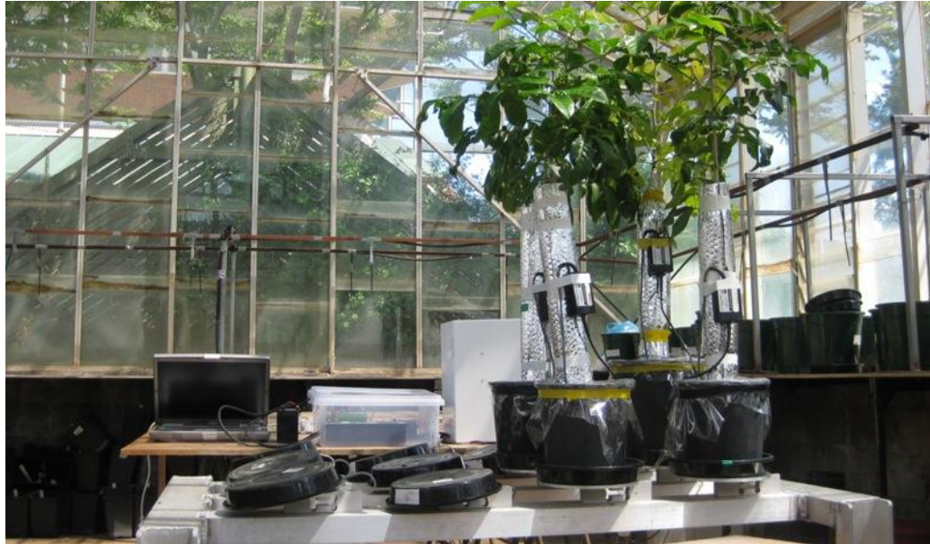
Figure C.1: Pot plants with installed sap flow gauge placed on mini lysimeter
