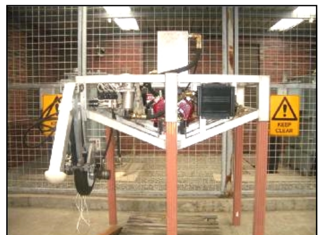
Fig 16. Front view of Hydrobug body showing mounted hydraulic ‘powerpack’ & prototype leg
