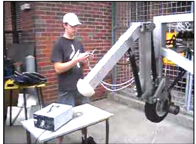
Fig 15. Prototype leg & wheel of the Hydrobug
