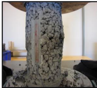
Figure 4.12 The gradually developed crack in the permeable concrete specimen with high porosity
