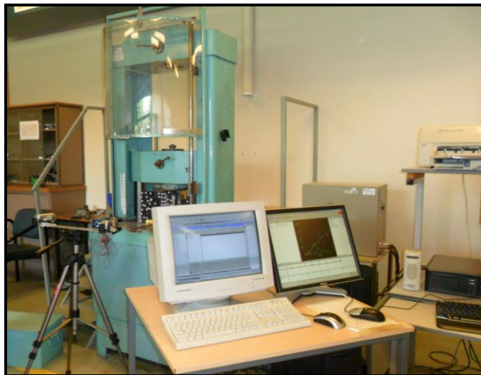
Figure 3.8 The strain measurement set-up using photogrammetry technology
