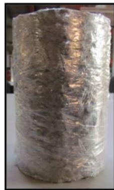
Figure 3.12 Permeable concrete specimen wrapped with cling wrap
