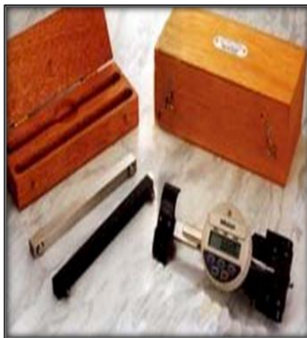
1. DEMEC with digital indicator
