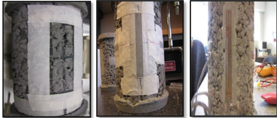
Figure 3.7 Steps in preparing and fixing the strain gauge onto the permeable concrete samples
