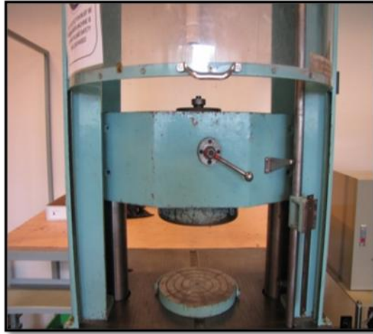
Figure 3.4 An 500kN Avery machine used for the compression strength test
