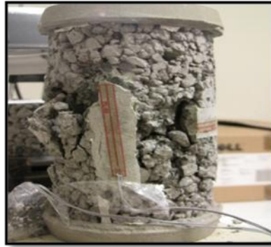
Figure 4.11 The sudden crack in the permeable concrete specimen with low porosity
