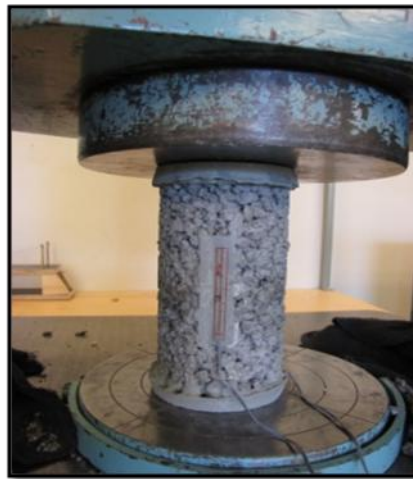
Figure 3.5 The sample's central location in the machine during the test
