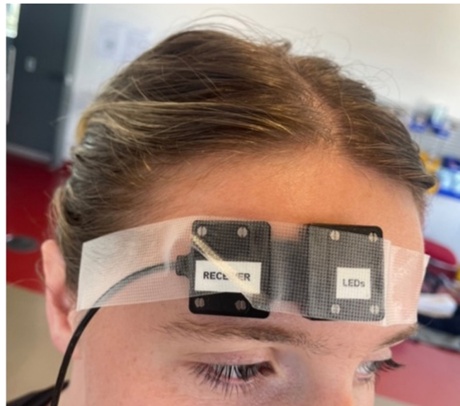
Fig. 3. Sensors consisting of 3 light-emitting diodes were placed approximately 2 cm above the right eyebrow and continuously recorded data whilst students completed high-acuity scenarios (Informed consent was obtained from the student in the photo.).
