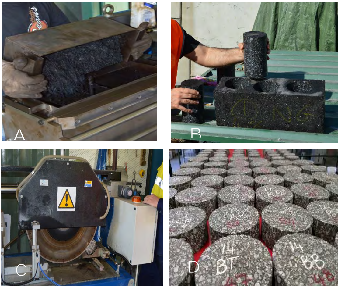
Figure: 4.13 A) Placing asphalt mix in the shear box compactor. B) Coring specimens from slabs. C) Cutting specimen to the required sizes. D) Prepared specimens
