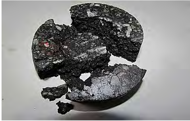
Figure: 6.14 Rapid collapse failure pattern for the Semi-confined 50/ 100 mm C170 test
