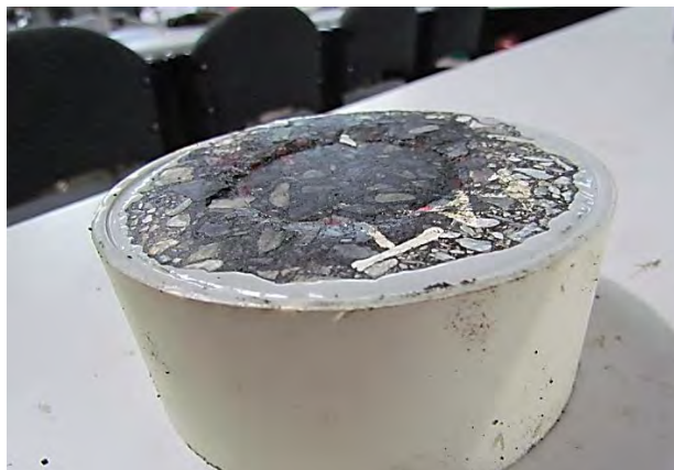
Figure: 6.21 Failure pattern for the CDCT confined 50/ 100 mm multigrade
