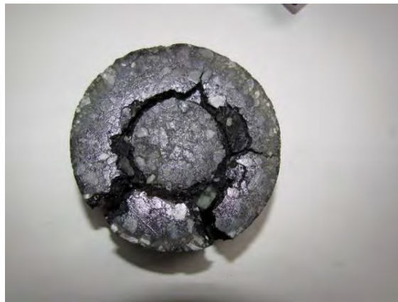
Figure: 4.9 Laboratory specimen punching when a simulated real traffic load was applied
