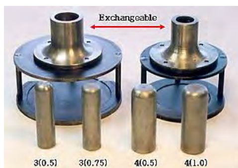
Figure 4.5 Test equipment for 150 mm specimens (left) and 100 mm (right) with replaceable loading-head holders (Doh et al. 2007)
