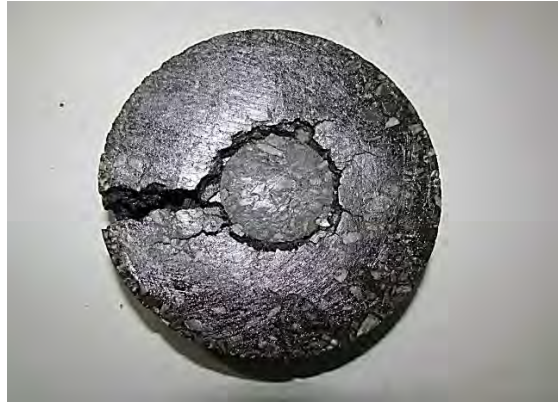
Figure: 6.10 Failure pattern for the Semi-confined 50/ 150 mm multigrade SCDCT tests
