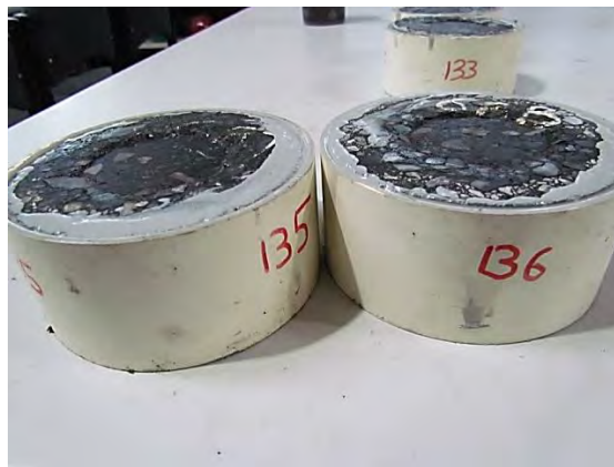
Figure: 6.30 Failure pattern for the CDCT confined (2.5 mm) 50/ 100 mm C170
