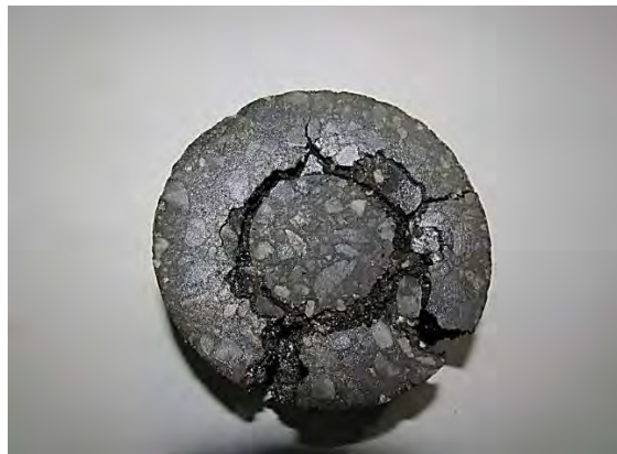
Figure: 6.6 Failure pattern for the Semi-confined 50/ 100 mm multigrade SCDCT tests
