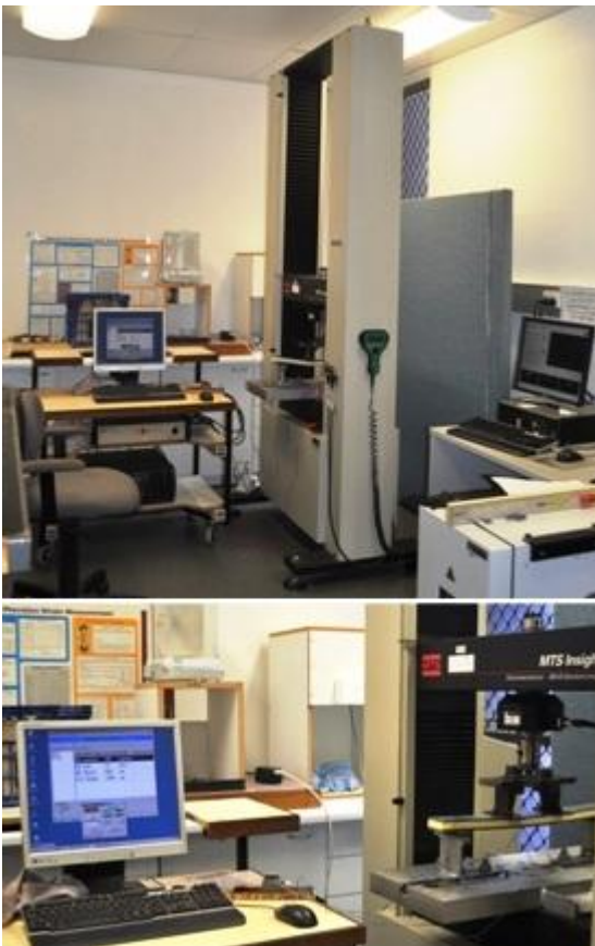
Fig. 3. Testing set-up for four point bending test
