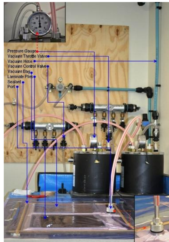
Fig. 2. The equipments for vacuum bagging process
