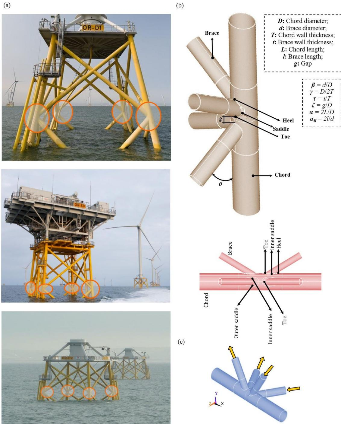
Fig. 1 (a) Multi-planar tubular KK-joints in OWT jacket substructures, (b) Geometrical notation for a multi-planar KK-joint and (c) Studied axial loading condition
