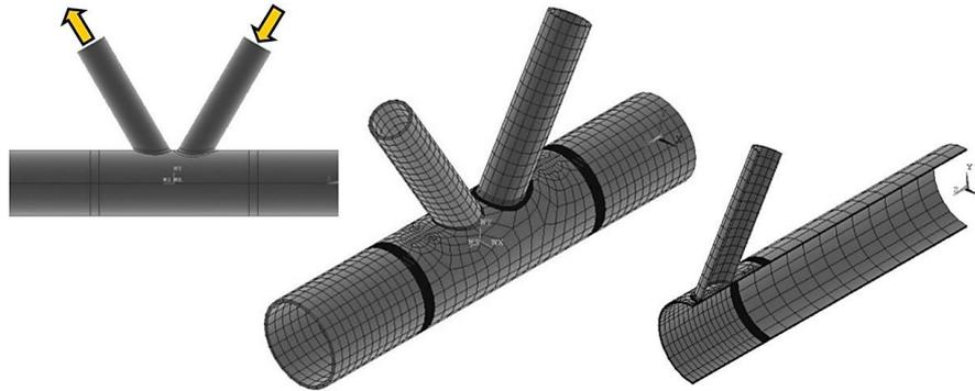
Fig. 7 Validating FE model generated for the comparison of the results with HSE OTH 354 (1997) experimental measurements
