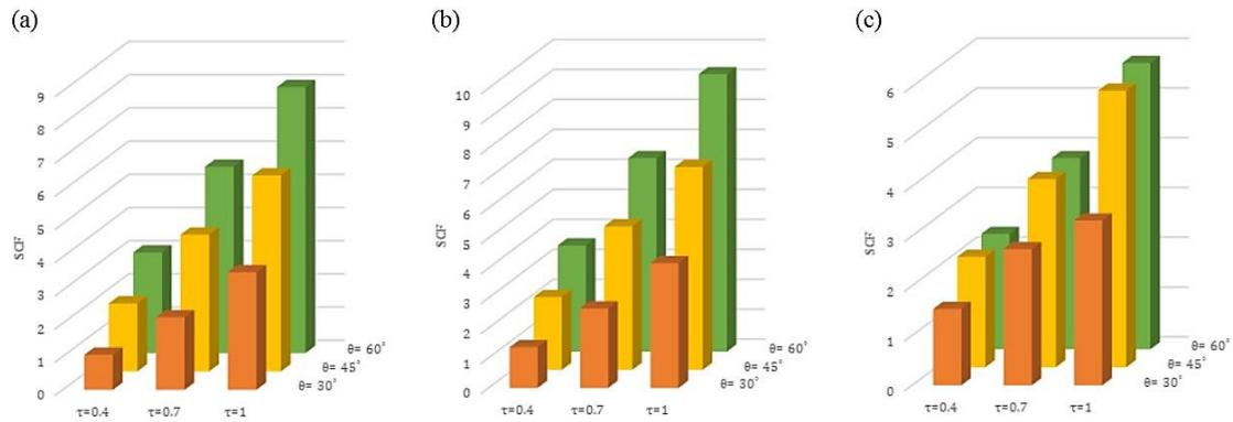
Fig. 9 The effect of the  $\tau$  on the SCF values and its interaction with the  $\theta$  ( $\beta = 0.3$ ,  $\zeta = 0.4$ ,  $\gamma = 18$ ): (a) Inner saddle position, (b) Outer saddle position and (c) Toe position
