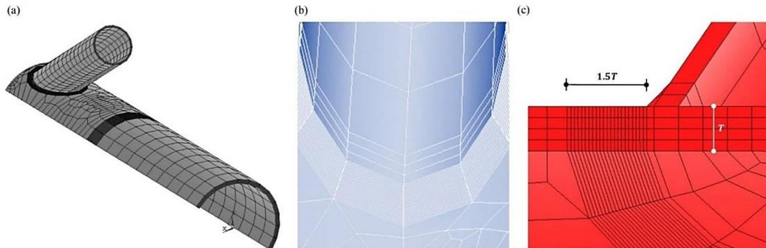
Fig. 5 Generated mesh by the sub-zone scheme: (a) One quarter of the joint under the axial loading condition, (b) Weld profile and extrapolation region and (c) Regions adjacent to the brace-to-chord intersection
