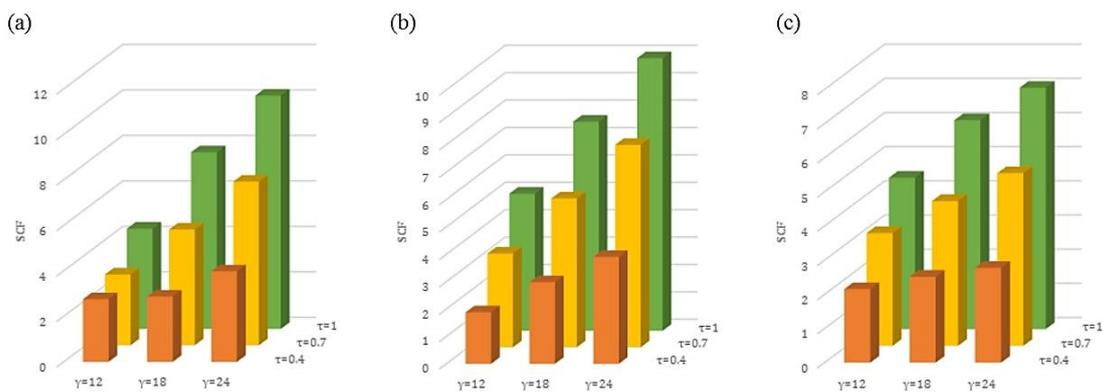
Fig. 10 The effect of the  $\gamma$  on the SCF values and its interaction with the  $\tau$  ( $\theta = 60^\circ$ ,  $\zeta = 0.2$ ,  $\beta = 0.3$ ): (a) Inner saddle position, (b) Outer saddle position and (c) Toe position
