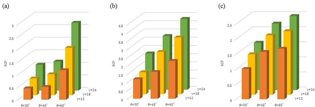
Fig. 12 The effect of the  $\theta$  on the SCF values and its interaction with the  $\gamma$  ( $\zeta = 0.4$ ,  $\beta = 0.5$ ,  $\tau = 0.4$ ): (a) Inner saddle position, (b) Outer saddle position and (c) Toe position
