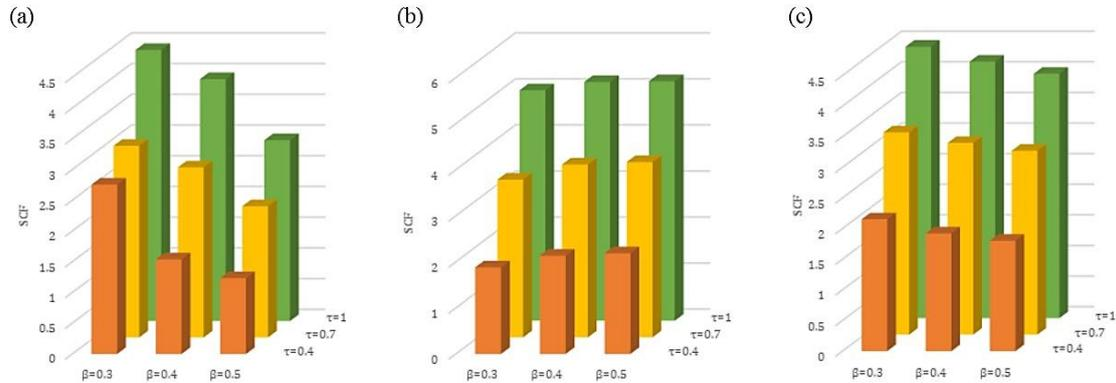
Fig. 8 The effect of the  $\beta$  on the SCF values and its interaction with the  $\tau$  ( $\theta = 60^\circ$ ,  $\zeta = 0.2$ ,  $\gamma = 12$ ): (a) Inner saddle position, (b) Outer saddle position and (c) Toe position
