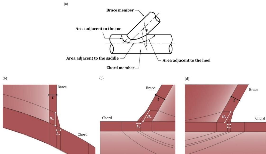
Fig. 2(a) Definition of the dihedral angle, (b) weld dimensions at the saddle position, (c) weld dimensions at the toe position and (d) weld dimensions at the heel position
