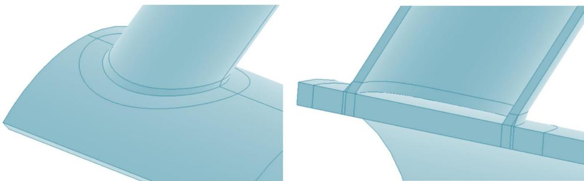
Fig. 3 The weld profile generated for a sample joint model ( $\beta = 0.4$ ,  $\gamma = 12$ ,  $\tau = 0.7$ ,  $\theta = 45^\circ$ )
