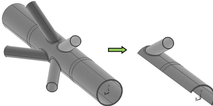
Fig. 4 One quarter of the entire multi-planar tubular KK-joint required to be modeled under studied axial loading condition
