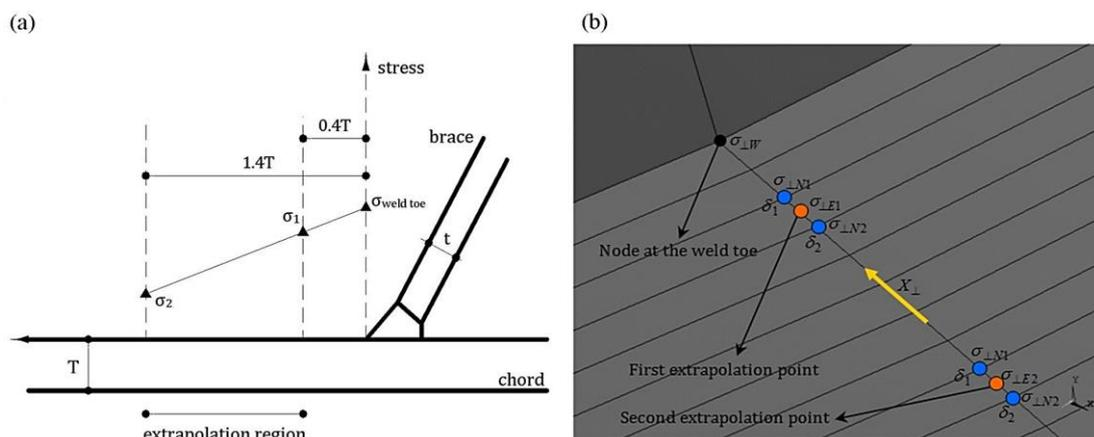
Fig. 6 (a) Extrapolation method according to IIW XV-E (1999) and (b) Required interpolations and extrapolations to extract the HSS value at the weld toe
