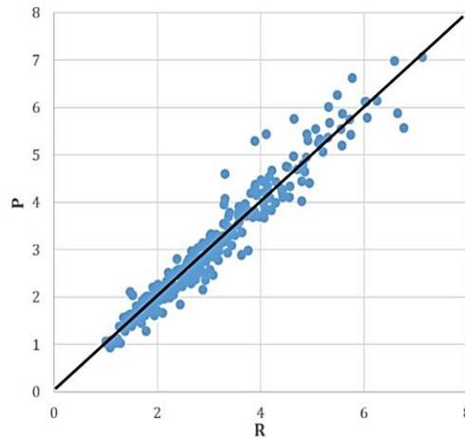
Fig. 13 Comparison of 243 SCF values calculated by the proposed equation for the toe position (Eq. (15)) with the corresponding SCF values extracted from the FE analysis (P: SCF value predicted by the equation, R: SCF value recorded from FE analysis)
