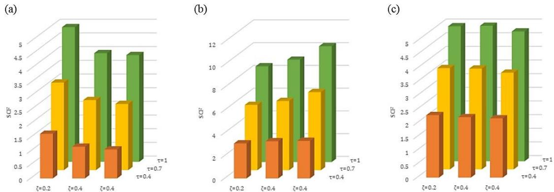
Fig. 11 The effect of the  $\zeta$  on the SCF values and its interaction with the  $\tau$  ( $\theta = 45^\circ$ ,  $\gamma = 24$ ,  $\beta = 0.5$ ): (a) Inner saddle position, (b) Outer saddle position and (c) Toe position
